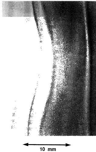
Figure 23. Synchronized helical flow in adjacent plumes, 'light field'. \text{NH}_4\text{Cl} -70 wt % \text{H}_2\text{O} , at a mean height of ca. 70 mm above growth front after 60 min.
